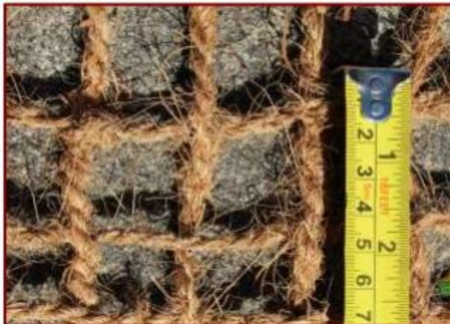
Coir geo-textiles specifications: Grade I- 400g/m 2
